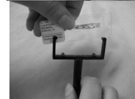
Place 1x2 inch clear box, 1x2 inch zip top bag, or a prepared slide in the slide holder. If using the clip, place the object in the clip.
