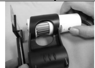
The focus wheel should face downward and be in the center opening in the camera holder.
