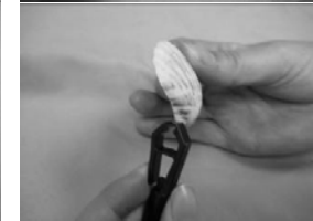
Place 1x2 inch clear box, 1x2 inch zip top bag, or a prepared slide in the slide holder. If using the clip, place the object in the clip.
