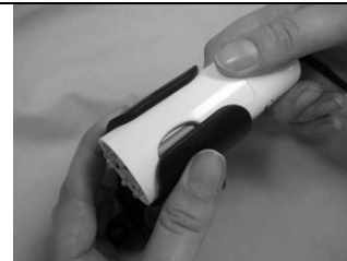
Rotate the Dlite 180 degrees by twisting the Dlite in the holder.
